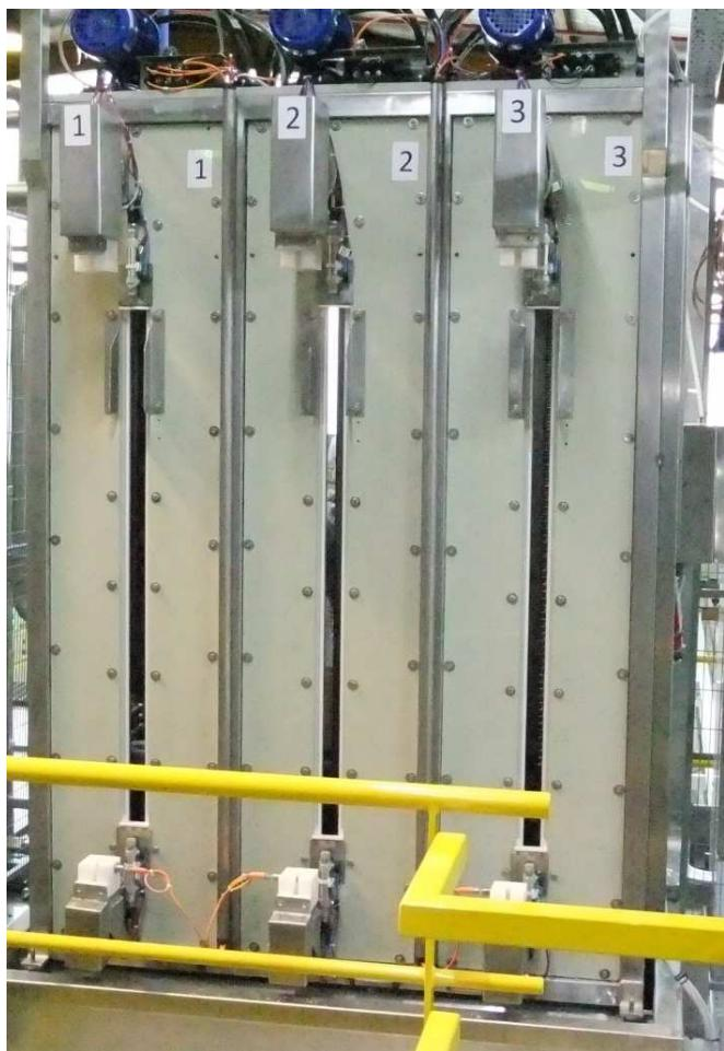
Machine completely in stainless steel AISI 304, suitable for vertical washing of a squeegees of one colour.
