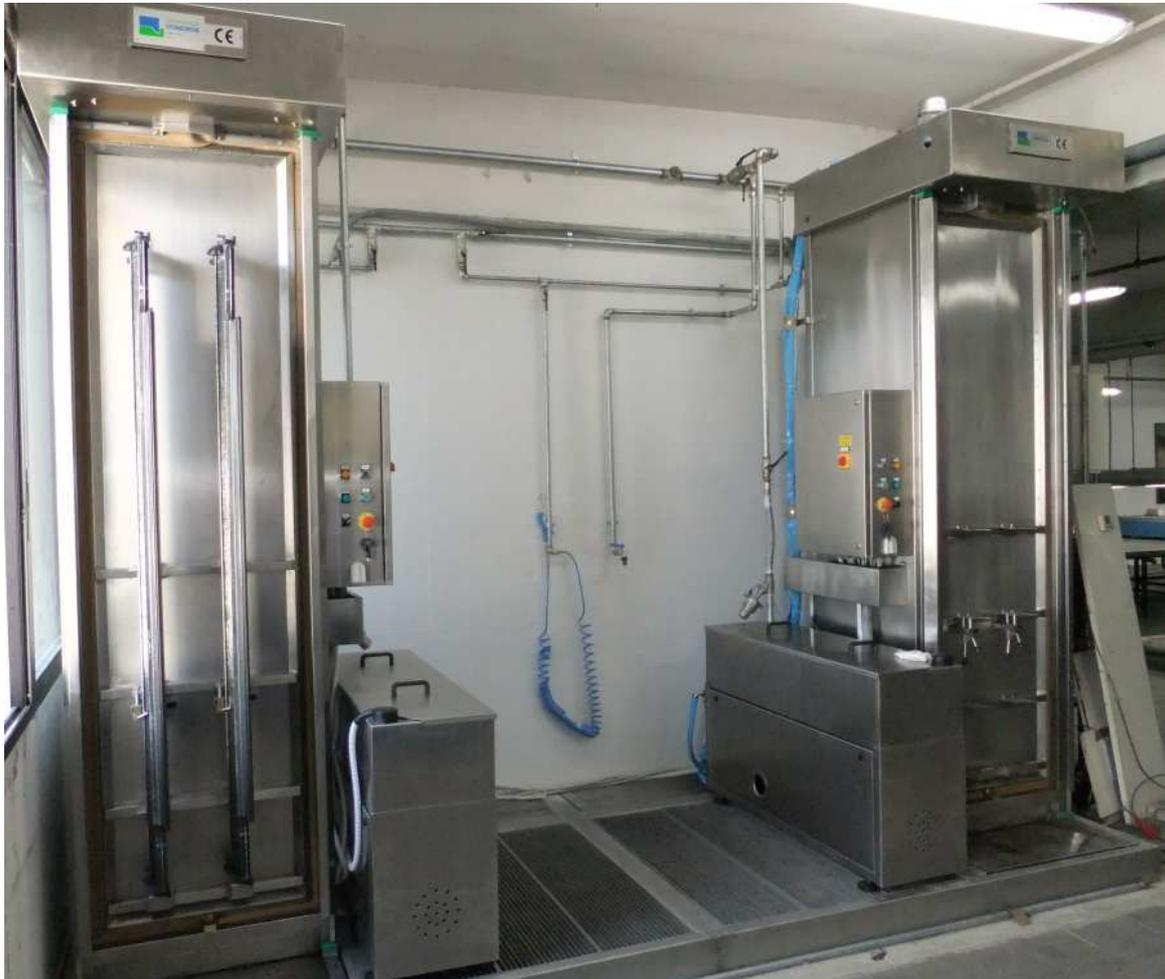
The machine MONOVER , made of stainless steel AISI 304, can wash and partial dry vertically a squeegees of one colour and the same time can collect the squeegees of the second colour.
