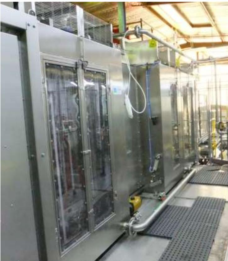
With movable nozzles, washing and rinsing sections.
